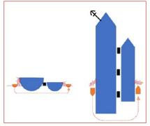
2. TO USE APPROVED BASKET & APPROVED CRANE FOR PERSONNEL TRANSFER. MAJORITY OF OUR SHIPS CAN PROVIDE SAFETY BASKET. IF BOTH SHIPS HAVE APPROVED CRANES - USUALLY USE CRANE FROM A SHIP WHICH HAS HIGHER FREEBOARD. CRANE RESTRICTIONS (MAX.ROLLING ANGLE, ETC.), CRANE OPERATOR EXPERIENCE, WEATHER AND PROPER PPE MUST BE CONSIDERED
